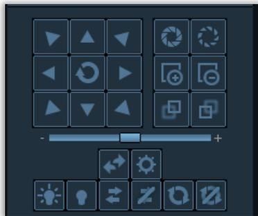
You can move PTZ to 8 directions through controlling direction buttons, and drag the slider to change PTZ moving speed, "-" is for slowing, "+" is for accelerating.
